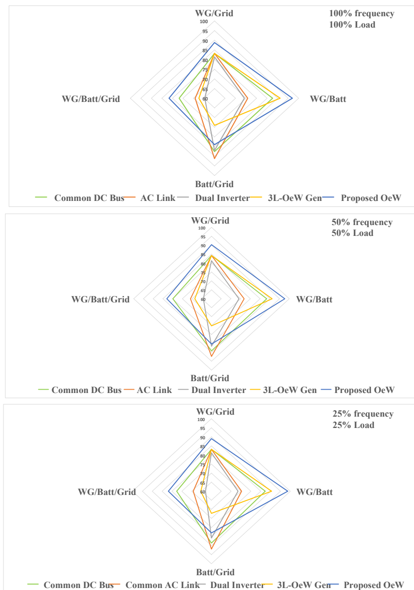
Fig. 4.28 Average efficiency comparison at 100% Load-frequency, 50% Load-frequency and 25% Load-frequency.
