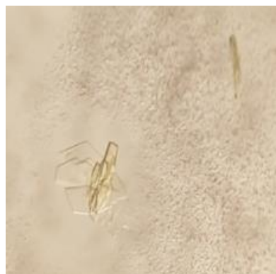
Figure 3.2.9.1.1: Crystals of AncFMO3-6. Crystals formed after 4 days at 20 °C in 0.1 M HEPES.Na pH 7.5; 5% (v/v) Isopropanol; 10% (w/v) PEG 4000 conditions.
