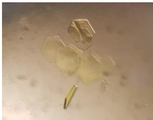
Figure 3.2.9.2.1: Crystals of AncFMO3-6, solubilized in CYMAL-6, formed after 2 days at 20 °C in 0.1 M Sodium Acetate pH 4.6 and 10% (w/v) PEG 4000 conditions.
