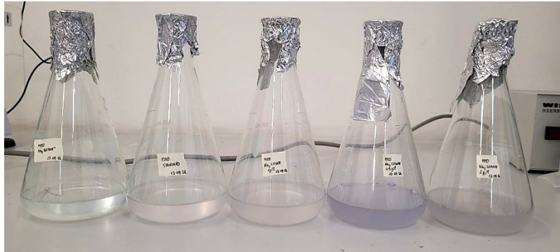
Figure 26 - Different concentration of \text{Na}_3 -citrate affects pyocyanin-derivative production.
