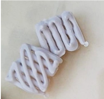
Figure 53 - 3D-printed scaffolds after functionalization with water-extracted pyocyanin derivative.
