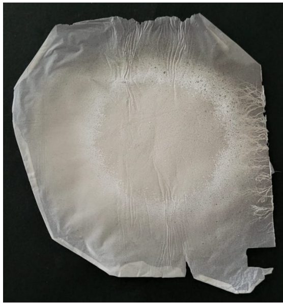
Figure 49 – Electrospun nanofiber with AgNPs incorporation
