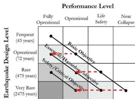
Figure 2.1. Seismic Performance Design Objective Matrix (modified from SEAOC Vision 2000, 1995).
